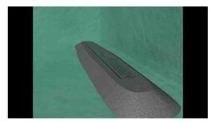
Pack you bedding material under and around your shower grate. Bedding material should then be scraped away from the shower grate to allow for tile and glue thickness. Insure the shower grate is plumb for aft and Left and Right
